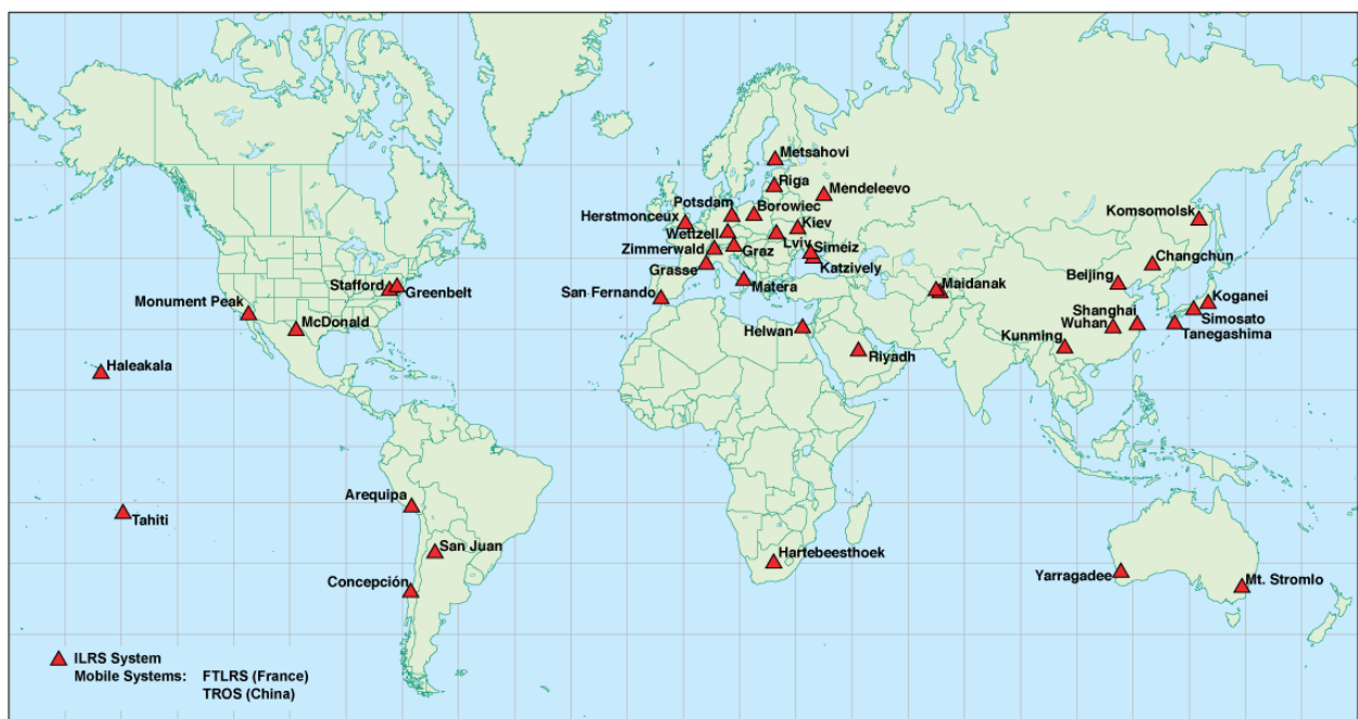
Fig. 1: The global network of SLR stations (status early 2007).
