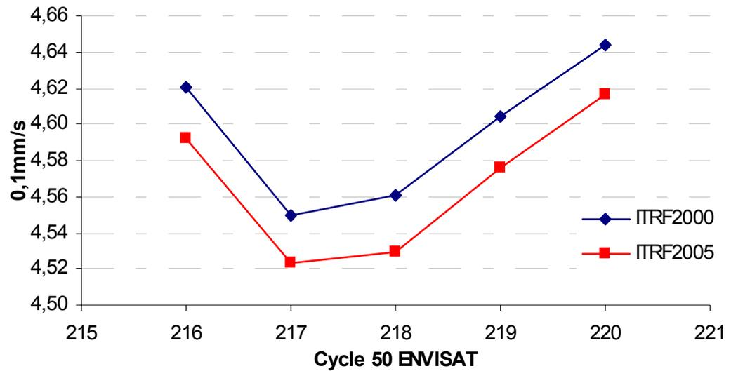
Fig. 5: DORIS fits for ENVISAT orbits based on SLR and DORIS tracking using ITRF2000 (blue line) and ITRF2005 (red line). In these tests by the CNES POD center, the DORIS performance is systematically improved with ITRF2005. The vertical scale ranges from 0.450 to 0.466 mm/s.
