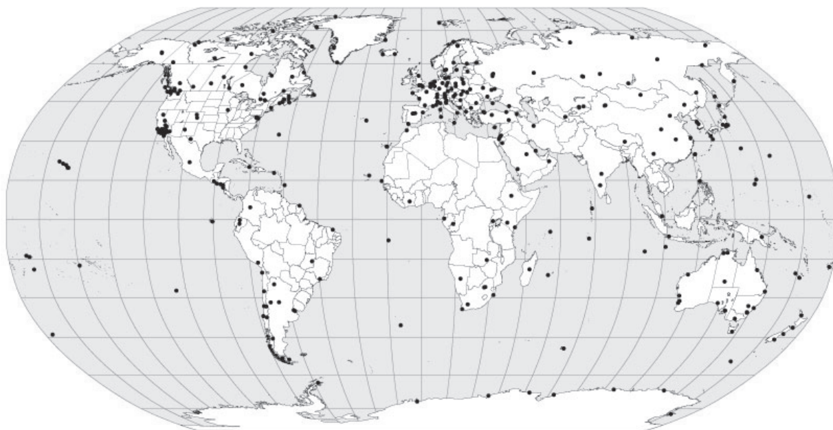
Fig. 1: IGS Global Tracking Network provides high quality tracking data used in support of diverse applications, including contributing to the realization of the ITRF.
