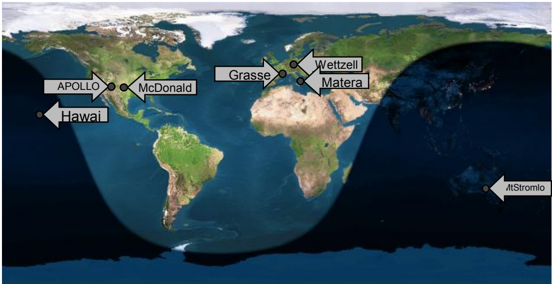
Fig. 2: The ILRS stations with lunar capability (status early 2008).
