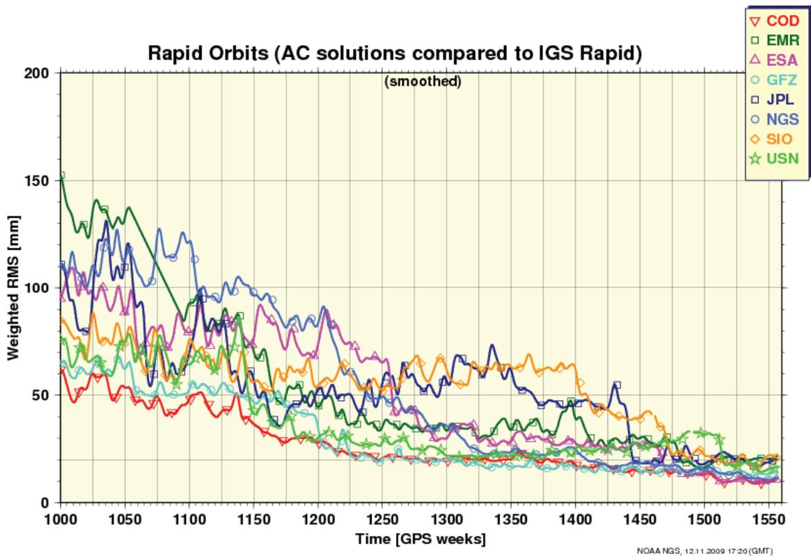
Fig. 6: Weighted RMS differences of all ACs' rapid orbits to the IGS rapid combined orbit.
