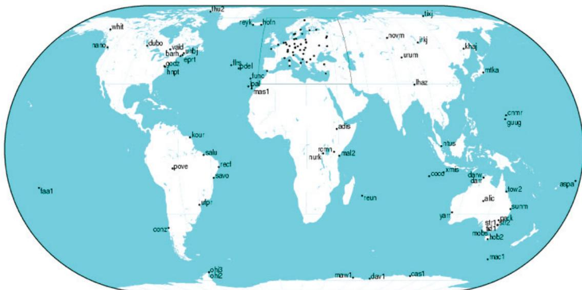
Fig. 3: IGS stations capable of tracking GLONASS satellites.
