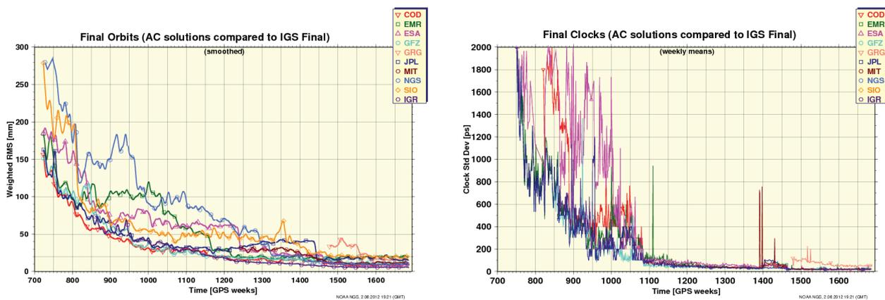
Fig. 2: (a) Weighted RMS differences of all AC's and IGS final orbits to the IGS final combined orbit. (b) Standard deviation of IGS final clock solutions.
