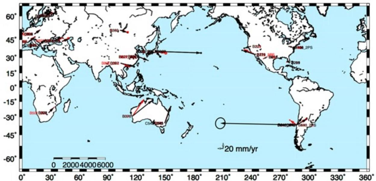
Fig. 1: Comparison of the velocity estimates for ITRF2014 (red vectors) and DTRF2014 (black vectors). DTRF2014 uses piecewise linear functions to represent postseismic motions and as a result some sites affected by large earthquakes have very large short term velocities. Sites shown here have separations  $< 10$  km and length uncertainty between VLBI and SLR sites less than 10 mm. Velocity differences between ITRF2014 and DTRF2014 make comparison of scale difference difficult.
