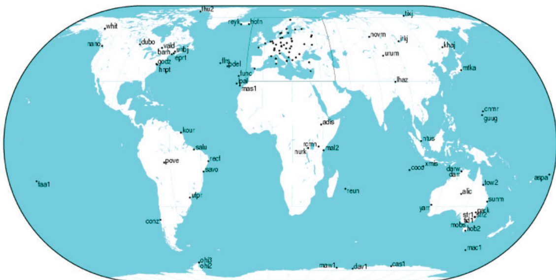
Fig. 3: IGS stations capable of tracking GLONASS satellites.
