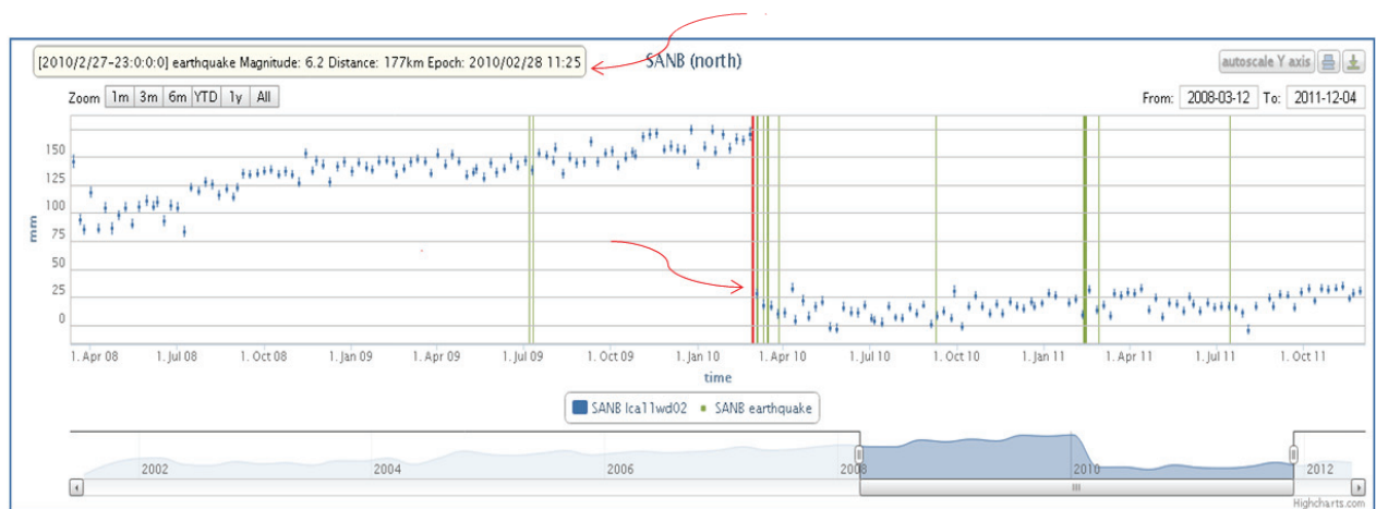
Fig. 2: Example of a position time series displayed with STCDtool: evolution of the North component of the DORIS station in Santiago with discontinuity due to the 2010 Chile Earthquake.
