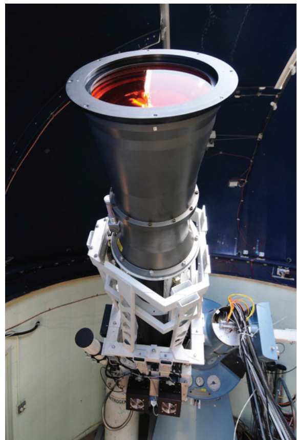
Fig. 10: The URAT "red lens" enabling accurate astrometry in a bandpass between R and I. In this picture the lens is seen without the shutter box.
