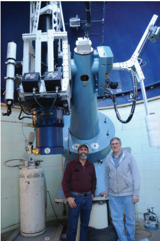
Fig. 9: The URAT telescope at NOFS with heads of instrument shops Mike DiVittorio (NOFS, left) and Gary Wieder (Washington DC, right). The movable counterweight is seen on the top right to keep the telescope mount in balance depending on liquid nitrogen fill level inside the dewar.
