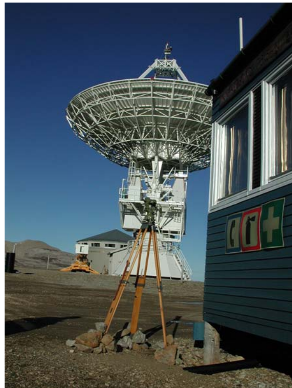
Fig. 2: Tripod stabilized with stones at NyAlesund Geodetic Observatory
