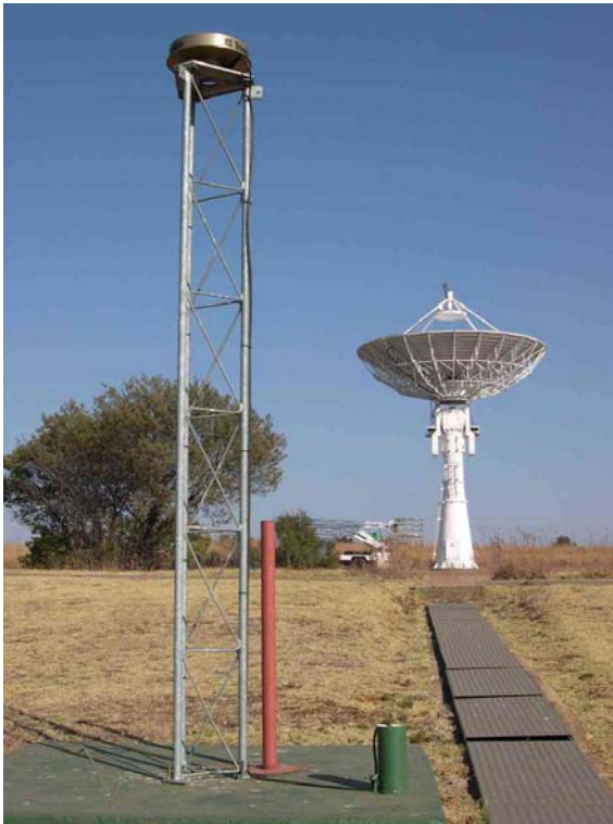
ChokeRing antenna of HARB IGS station
