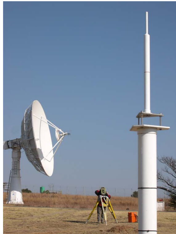
DORIS antenna on its pier
