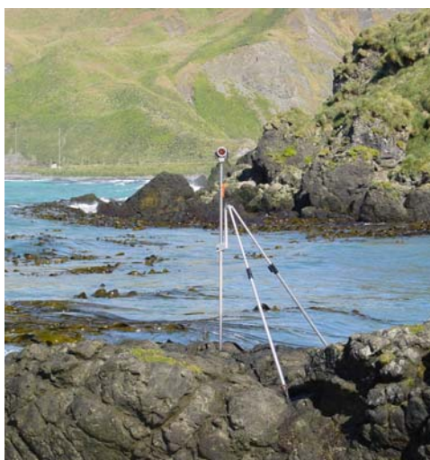
Figure 5: Fixed height prism pole for Total Station Levelling (TSL).
