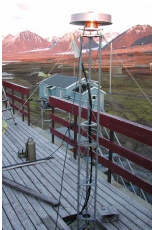
Figure 11: The GPS antenna mounted on the DORIS monument.
