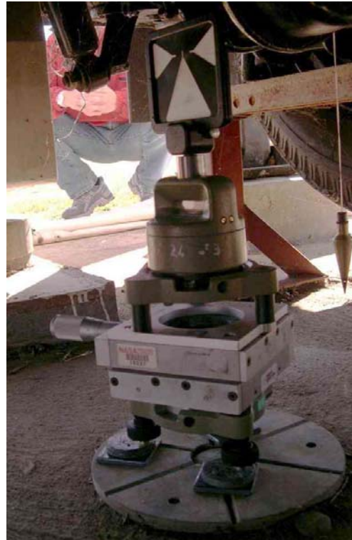
Eccentricity measurement above the brass ground mark (IGN method)
