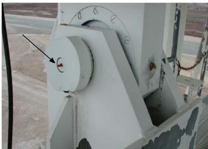
Figure 5: Target materialized by a pop rivet at the end point of the elevation axis.
