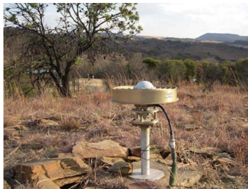
ChokeRing antenna of HRAO IGS station
