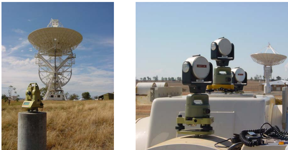
Figure 4: Left Leica TCA2003 Total Station. Right Leica Precision prisms with Tribrach and carriers (including plate bubble).
