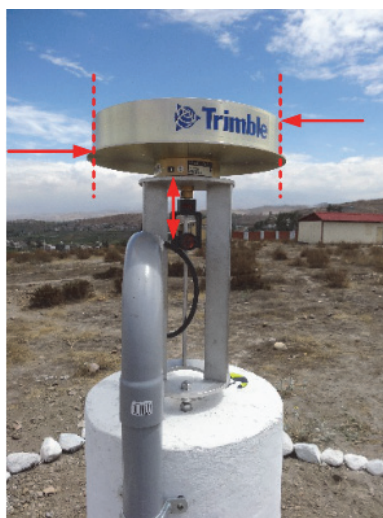
Figure 21: Determining antenna direction and distance
