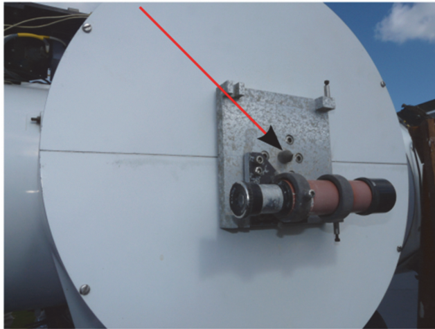
Figure 12: Piercing point on the horizontal axis at Herstmonceux SLR station.
