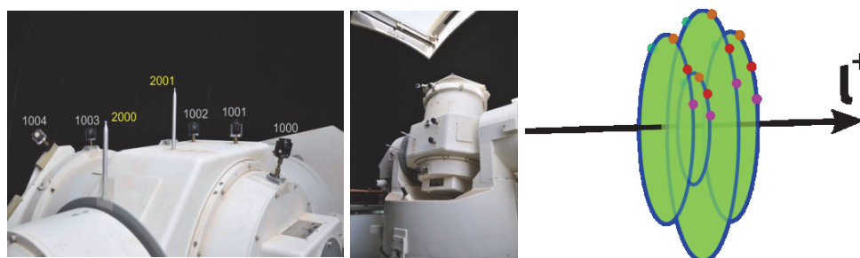
Figure 25: Surveyed points (2013 campaign) on MeO lunar laser at Grasse / Calern
