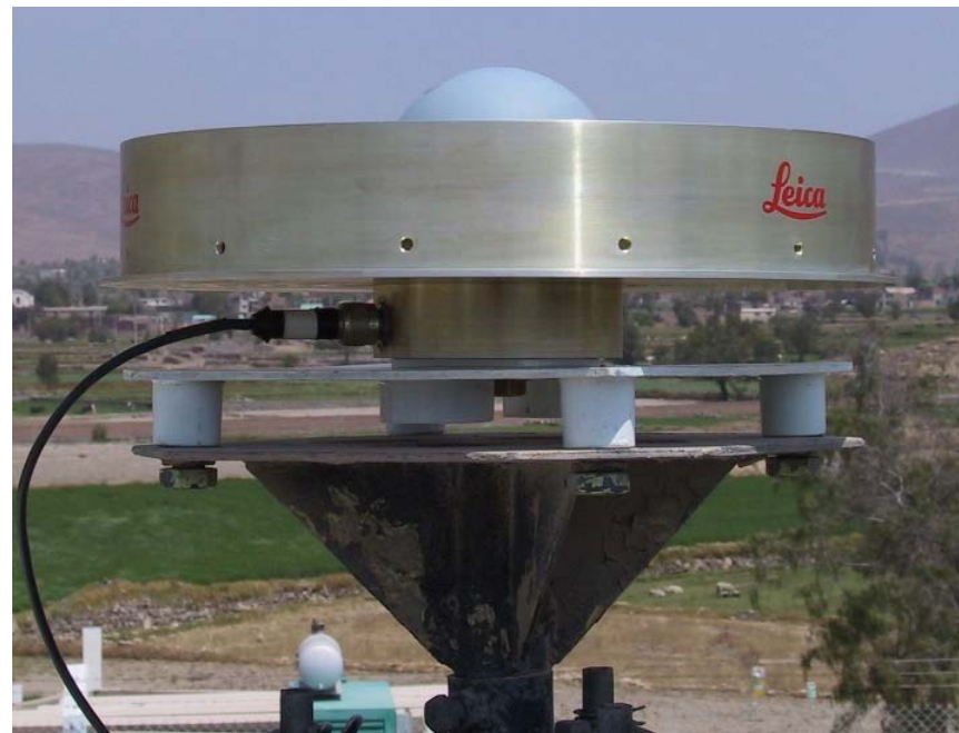
GPS survey using the forced centering interface
