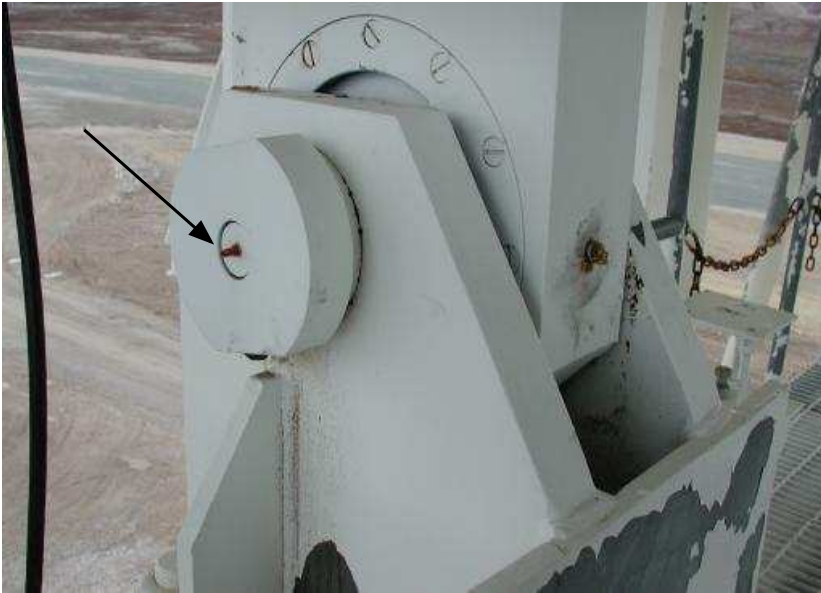
Figure 5: Target marker at end point of elevation axis (VLBI telescope).
